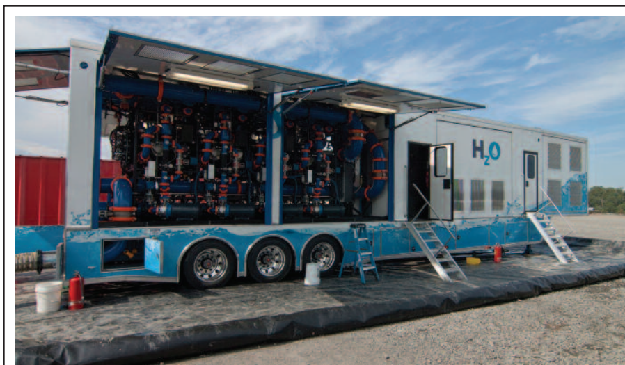
Hydrozonix LLC is expanding its fleet of EF80™ treatment units to service fracturing operations in the Permian Basin and the Marcellus Shale, with the company planning to build two units each quarter over the next two years, depending on market demand. Each EF80 unit can treat 80 bbl/minute during fracturing and post-frac flow back. The systems use the patented Ozonix™ oxidation process that incorporates ozone, hydrodynamic cavitation, and electro-chemistry for microbial control and scale inhibition.
