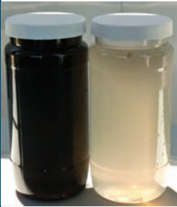
Samples taken before and after treatment of flowback water by the Hydrozonix EF80.
