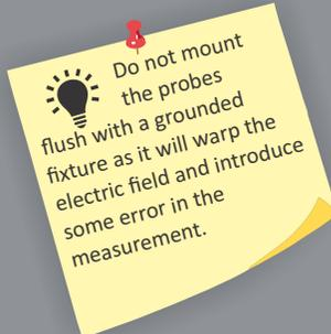
Dielectric thickness measurement works best with materials that have good control over their dielectric content. If batch to batch variation exists, recalibrate the probes with two samples of known thickness to teach the system the dielectric constant and probe to gap separation.
