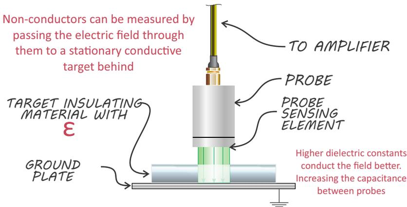
MTI's capacitance probes emit an electric field that passes through the insulating material, and the dielectric constant of the insulating material conducts that field. In order for the capacitive system to measure thickness it must account for different dielectric constants by going through a calibration with the material to be tested. As long as the dielectric constant of the material doesn't change then the calibration will remain consistent.
