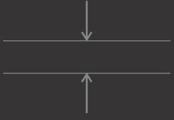
Placing a dielectric (non-conducting) material between two capacitance probes creates a three capacitor equivalent circuit.
