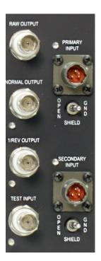
Select between primary and secondary input signals - Many engines have primary and secondary speed signals. Consequently, the TSC-4800A permits the selection of multiple input sources for each channel. Primary and secondary inputs are via three pin MS connectors where a full differential signal can be accepted.
