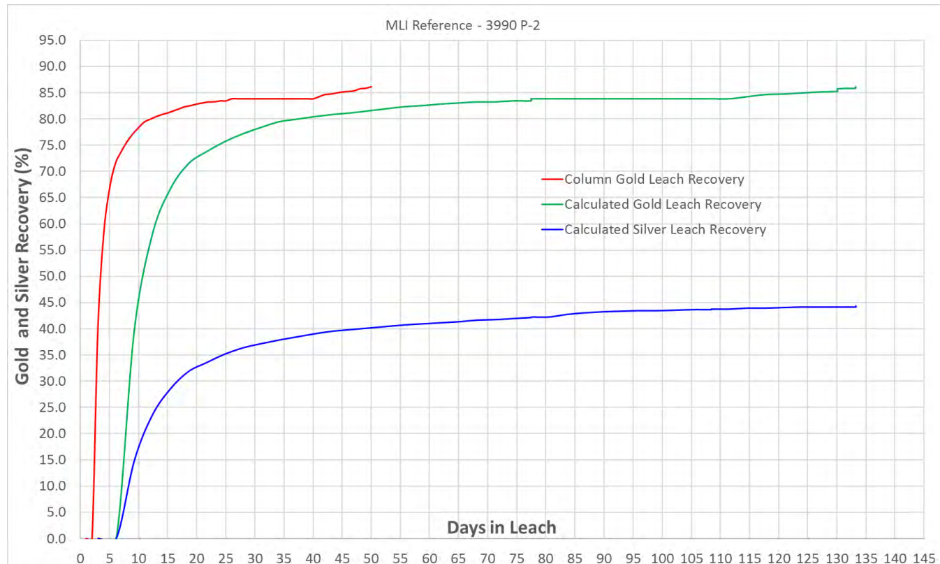
Figure 13.5 Column-Leach Rate Profiles, Bulk Sample BS-1, - 80% - 3 inch Feed
