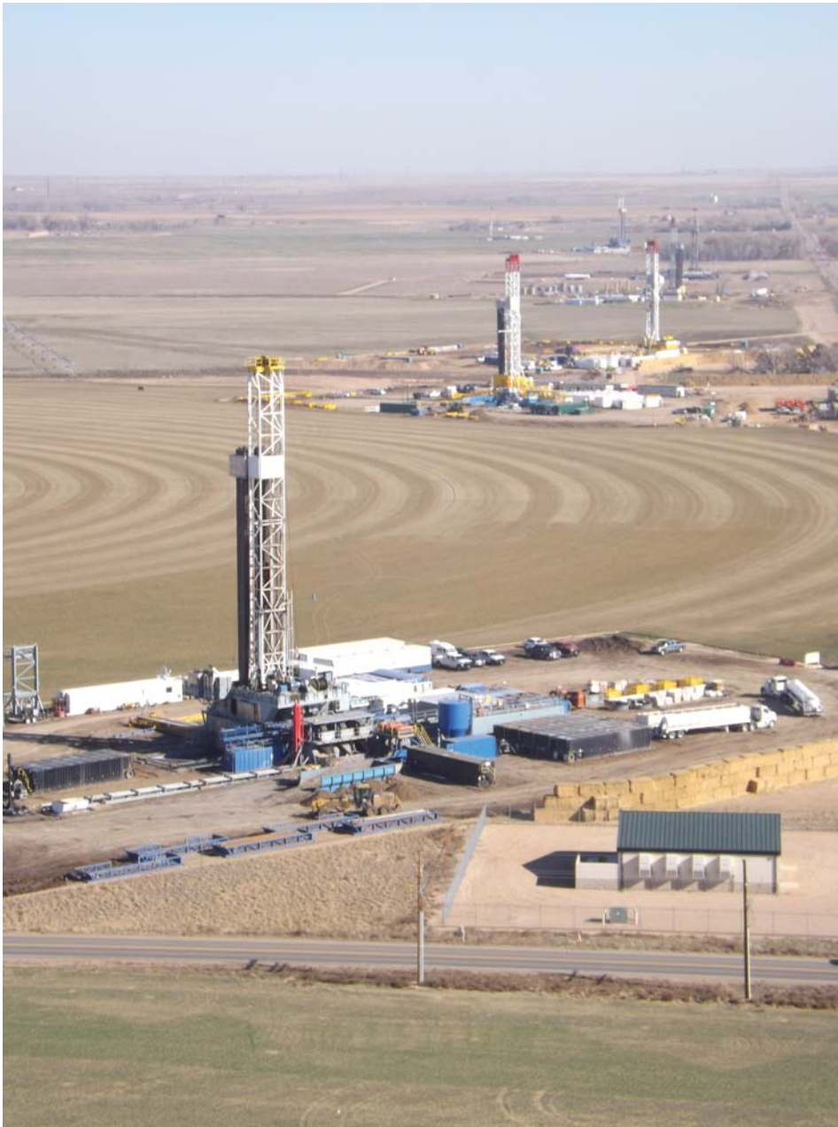
Wattenberg Field, Colorado - Seven drill rigs located within 4 miles of one another, drilling 8 to 16 wells per square mile for Niobrara and Codell Oil.
