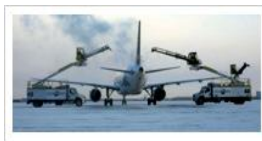
Figure 1: High Efficiency Deicing Trucks showing spray pattern.
