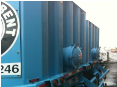
Figure 5: 21,000 gallon temporary storage tank
