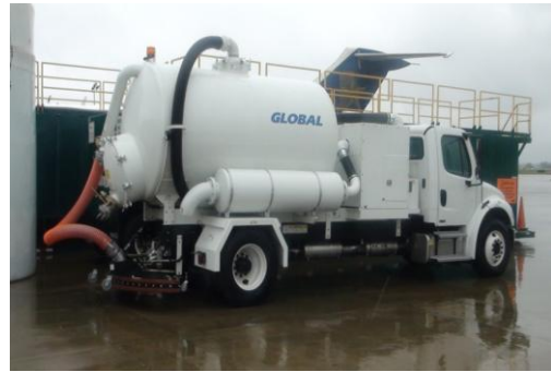
Figure 4: Global Ground Recovery Vehicle with 2,000 gallon tank
