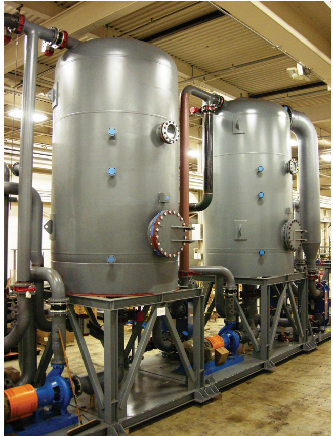
A Multistage CAST® (Controlled Atmospheric Separation Technology) distillation vessel under construction at ThermoEnergy Corporation's manufacturing plant in Worcester, MA.
