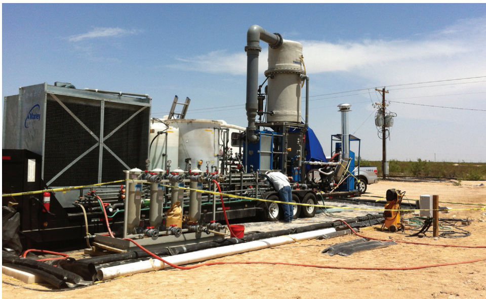
A ThermoEnergy TurboFrac 65 BPD pilot system is recycling produced water in the Permian Basin.
